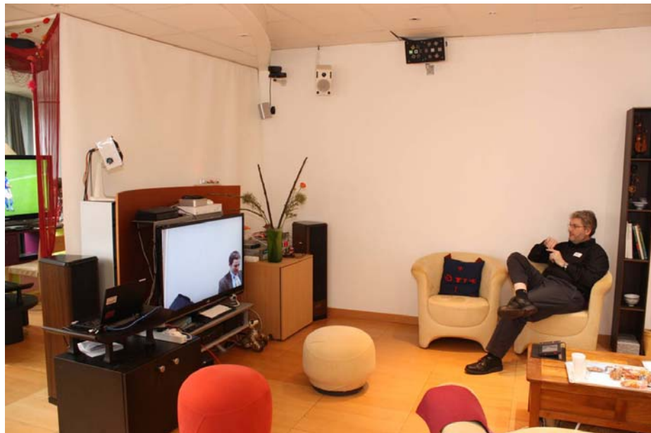
IRC base station (in centre of picture just below ceiling) communicating with terminal (above TV) for videoconferencing.
